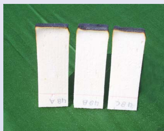
Fig.1-Photographs of RPUF samples incorporated with ATH: (a) before flammability test and (b) after flammability test
