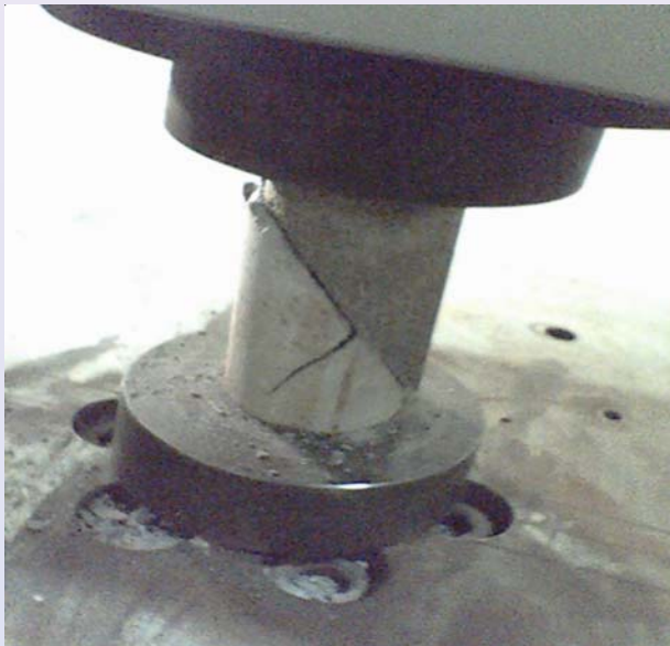
Fig.5-Polymer Modified Repair Material under Test
