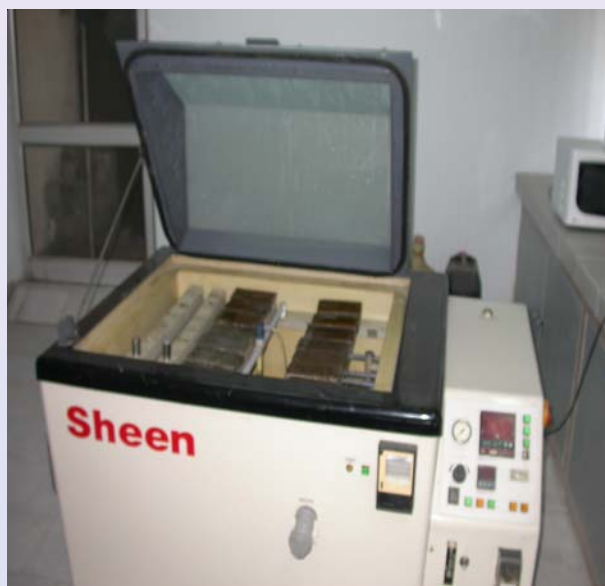
Fig.10-Coated panels with developed formulations under test.
