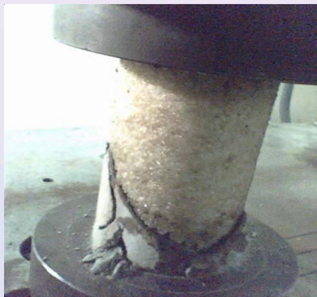
Fig.5-Polymer Modified Repair Material under Test
