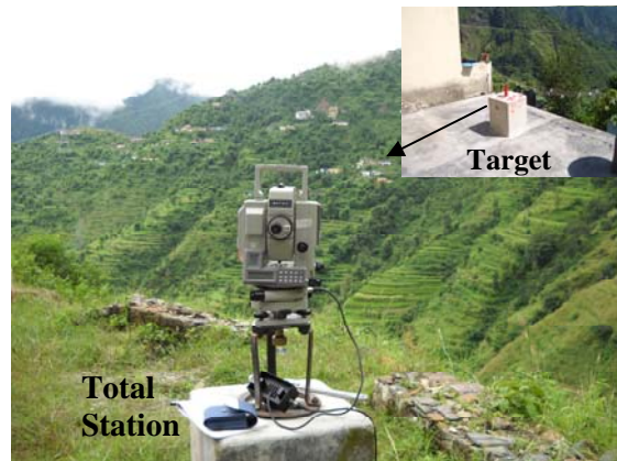
(a) Houses being monitored (a) and position of Total Station and target (b)
