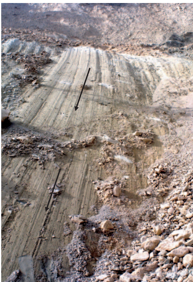
Fig. 3. Slip surface showing striations caused by sliding.
