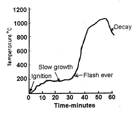
FIGURE 1. POSSIBLE COURSE OF A FULLY DEVELOPED BUILDING FIRE
