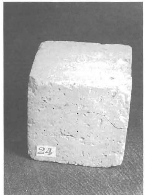
Fig. 9. Concrete cube having uncoated MS rebars (45 cycles).
