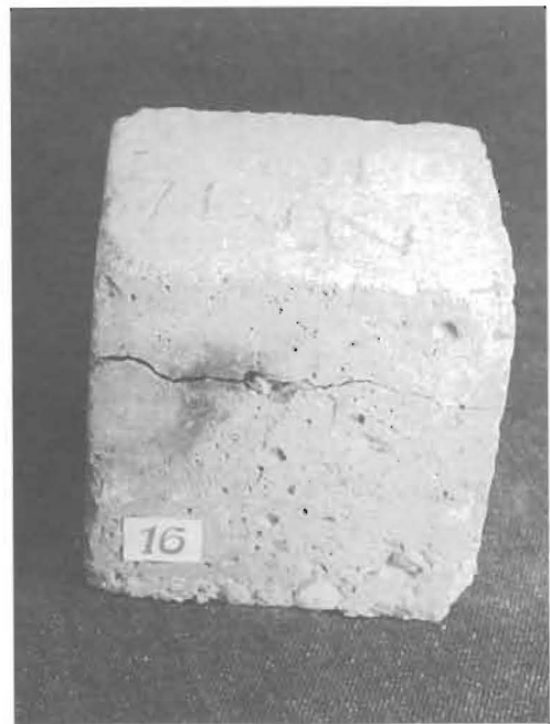
Fig. 13. Concrete cube having zinc-rich epoxy-coated MS rebars (80 cycles).
