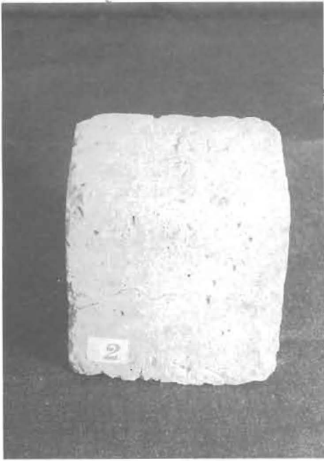
Fig. 10. Concrete cube having uncoated CRS rebars (50 cycles).
