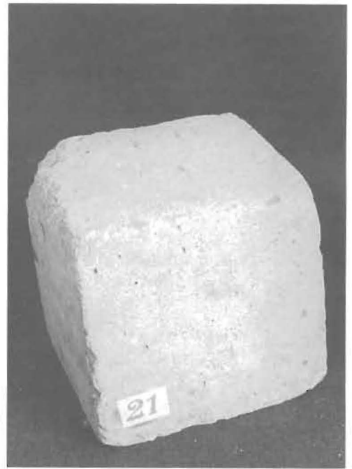
Fig. 16. Concrete cube having epoxy-coated MS rebars (80 cycles).
