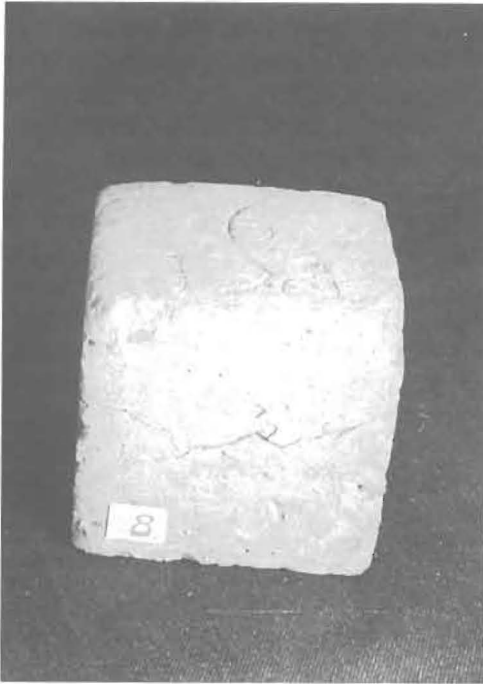
Fig. 14. Concrete cube having polyurethane-coated MS rebars (80 cycles).
