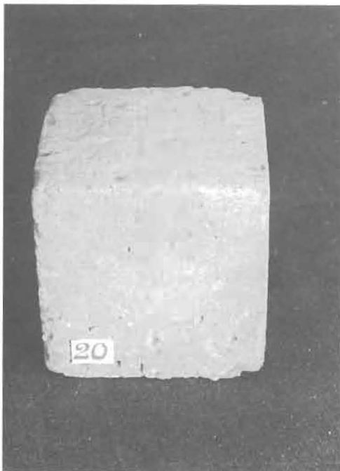
Fig. 15. Concrete cube having IPN-coated MS rebars (80 cycles).
