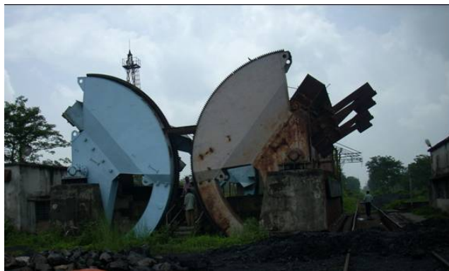
Figure 1 A wagon tippler used for unloading coal from the wagons.
