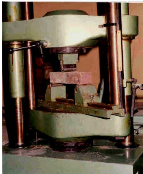
Fig.4:-Test set up for bond strength in flexure
