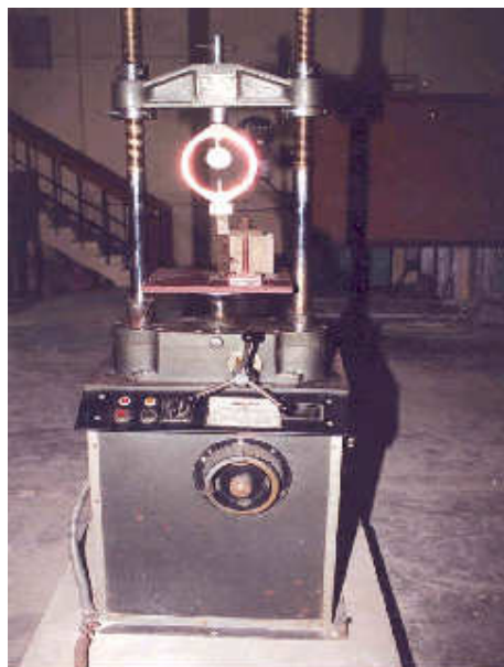
Fig.2: Test set up for bond strength (shear)
