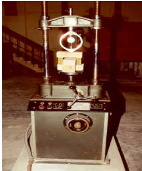
Fig.1: Test set-up for bond strength (in perpendicular direction)
