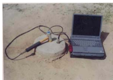
Fig.1. Low strain integrity test set-up
