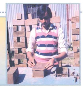
Application/Uses: For moulding of building bricks.
