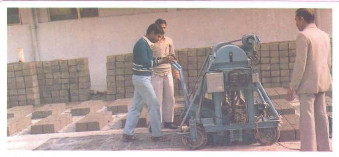
Application/Uses Suitable for casting solid and hollow concrete blocks with stone aggregates
