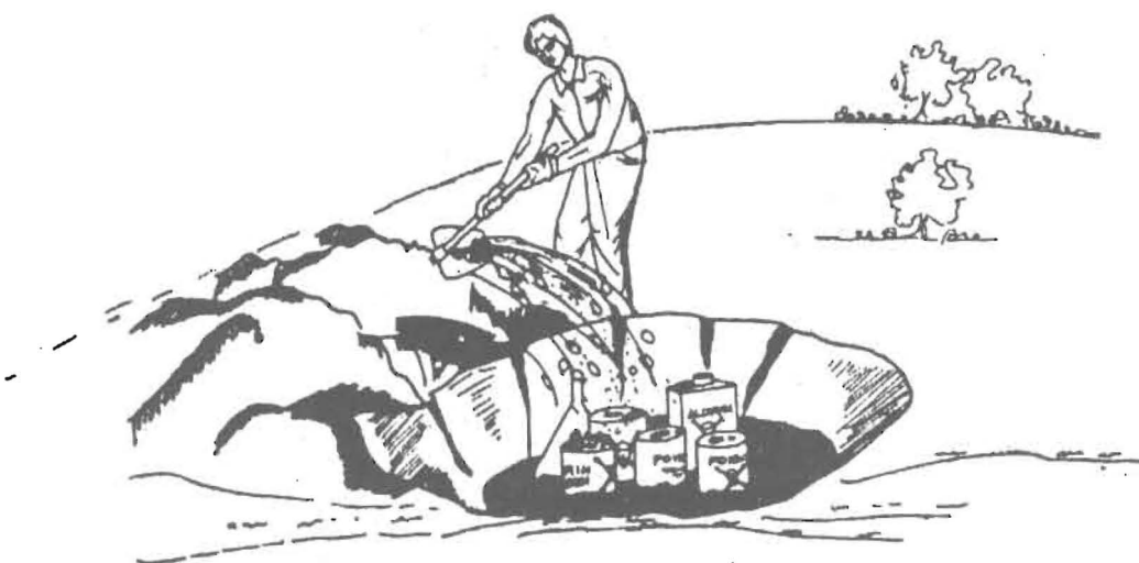
Fig. 4 Containers should be buried under the ground
