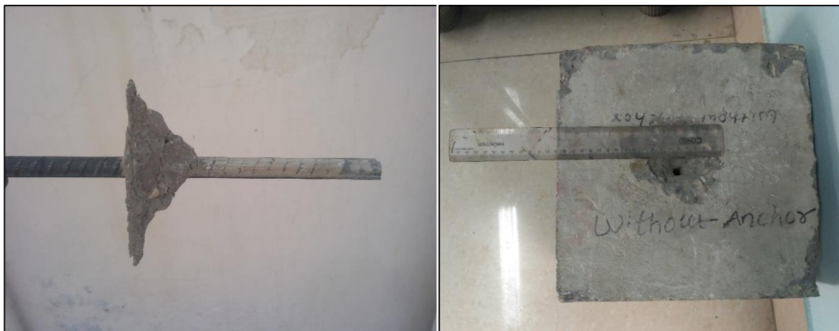
a) Bar portion after failure
