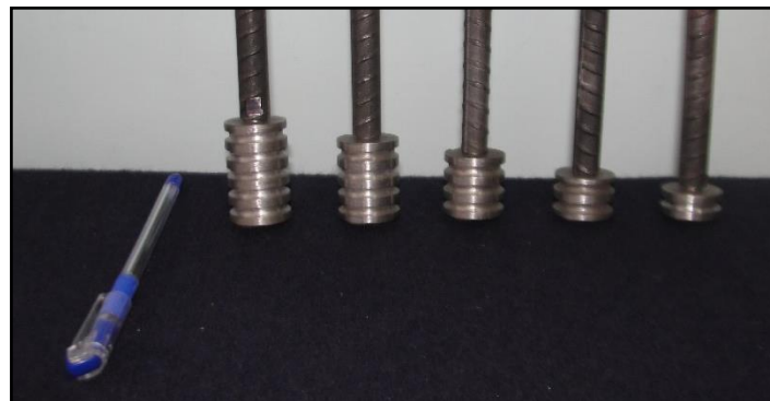
Figure 5.3: View of Groove mechanical anchor fixed to rebar
