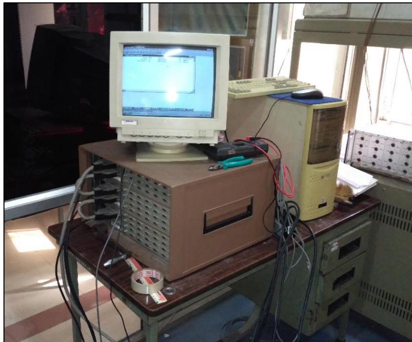
Figure 5.18: System with data acquisition for strain recording
