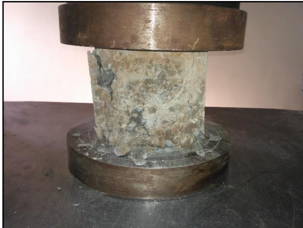
(a) Crack developed during compression testing
