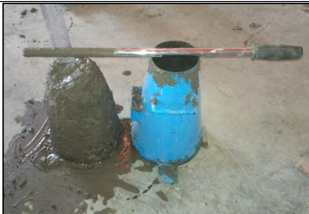
(a) Slump test of concrete
