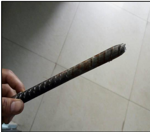
a) Fracture portion of bar
