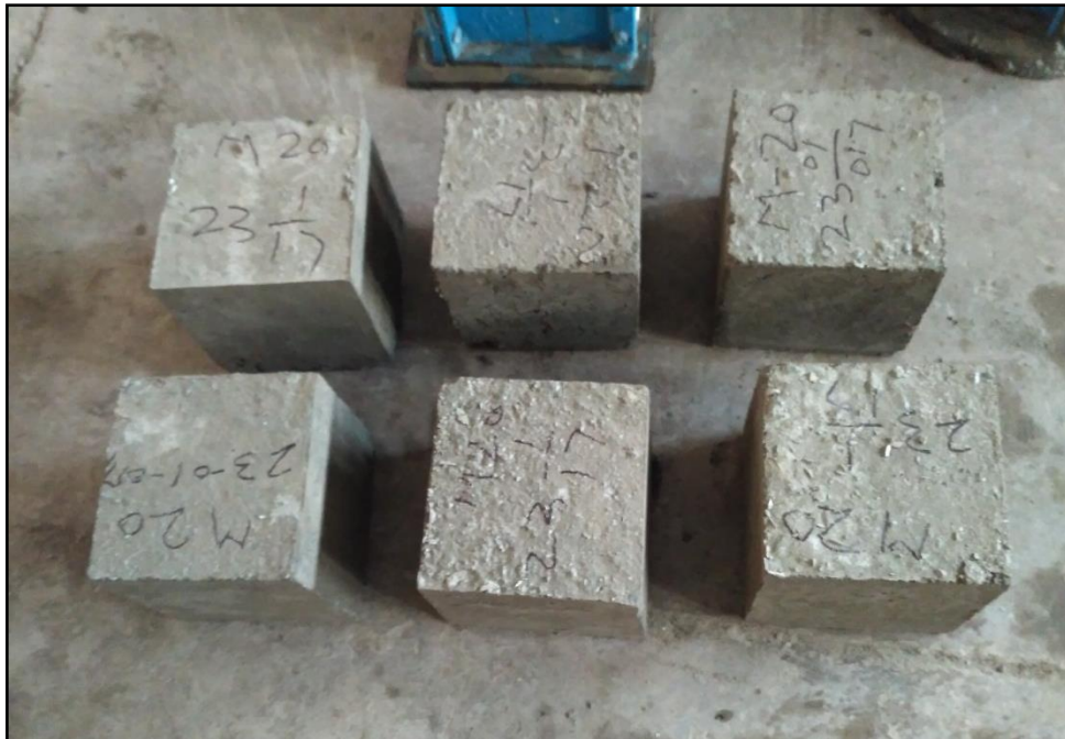
Figure 3.6: Concrete cube specimen for compression testing
