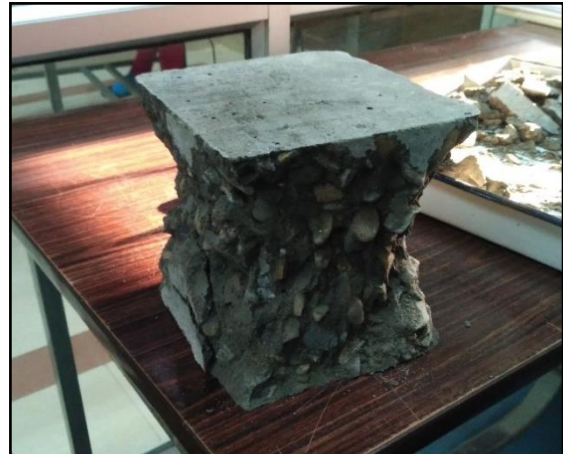
(b) Failure pattern observed
