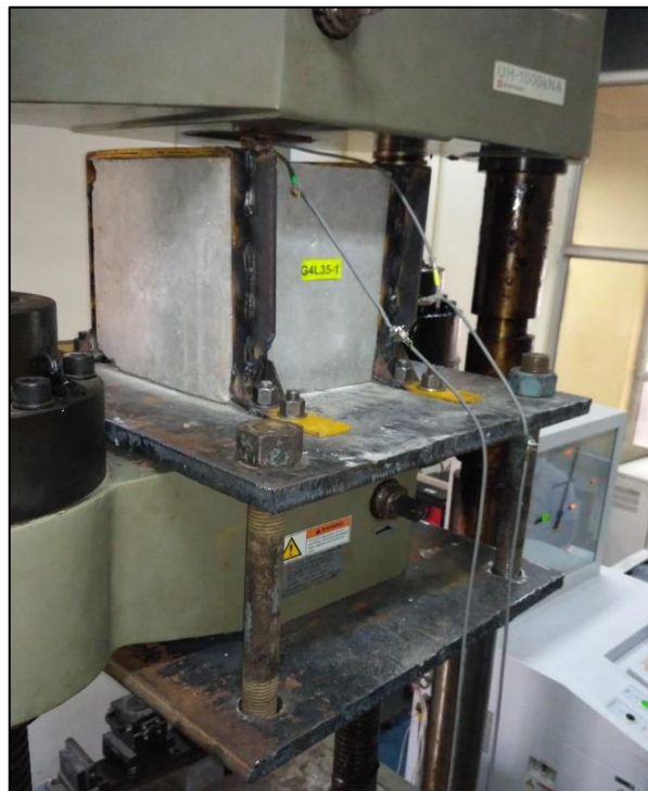
Figure 5.14: Test setup showing upper and lower plates fixed by bolting with UTM
