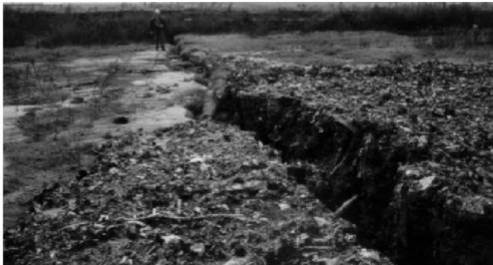
Fig. 1.3 Liquefaction of Sand at landfill site in Kobe, Japan (Bray et al., 1998)
