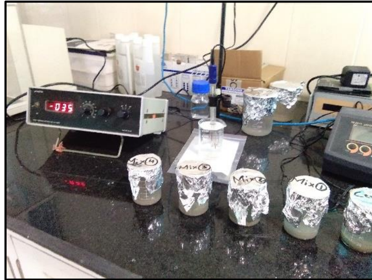
Fig. 3.25: The experimental setup for determining pH of blended mixes
