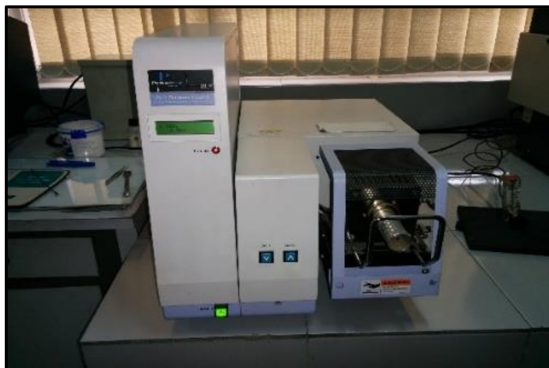
Fig. 3.15: TGA/DTA instrument for determining weight loss of a material
