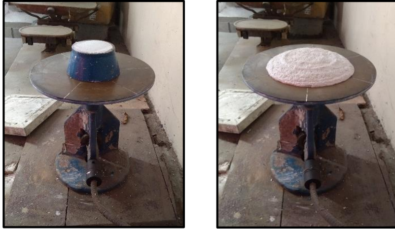
Fig. 3.19: Flow table for mortar flow
