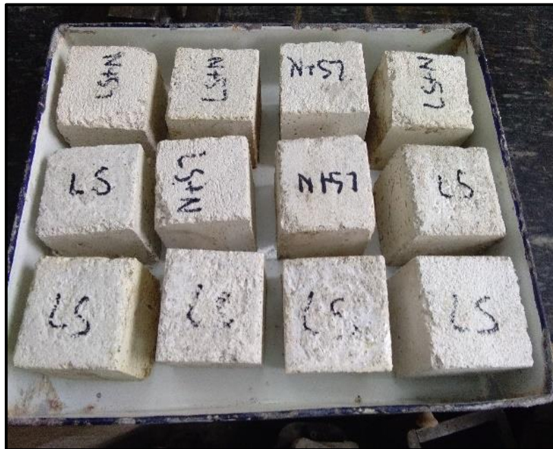
Fig. 3.20: Mortar cubes for lime reactivity
