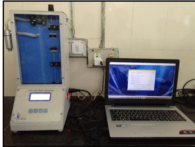
Fig. 3.12: The experimental setup of the automatic Blaine's apparatus
