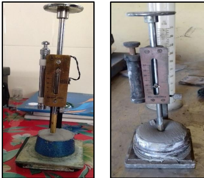
Fig. 3.17: The Vicat's apparatus for measuring consistency of cement
