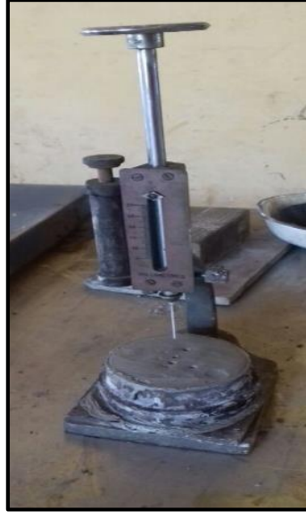
Fig. 3.18: Vicat's apparatus showing setting time of a blended cement
