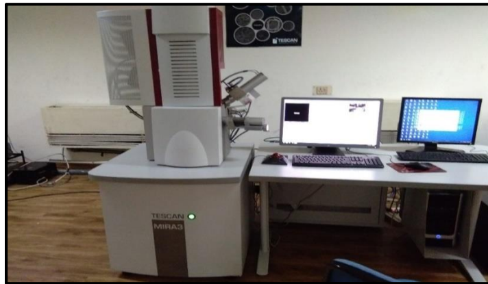
Fig. 3.14: Field emission scanning electron microscope for fractographic examination
