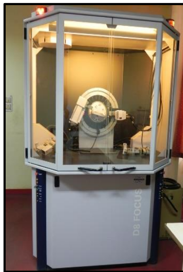
Fig. 3.13: The photographic view of X-ray Diffractometer
