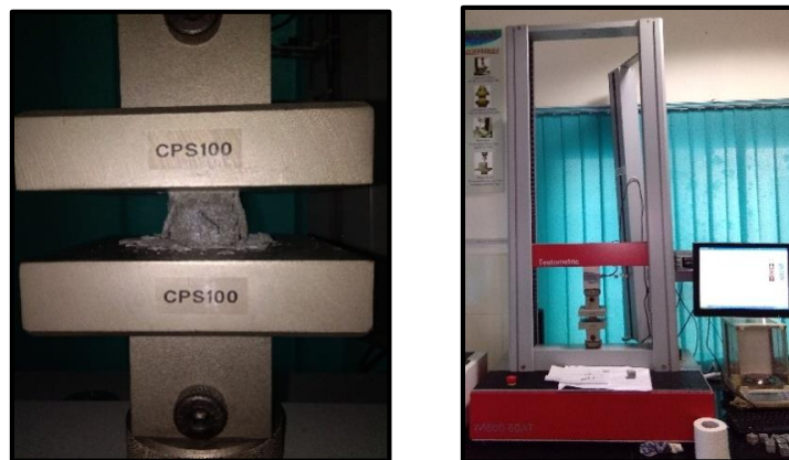
Fig. 3.27: Universal testing machine for compressive strength of paste
