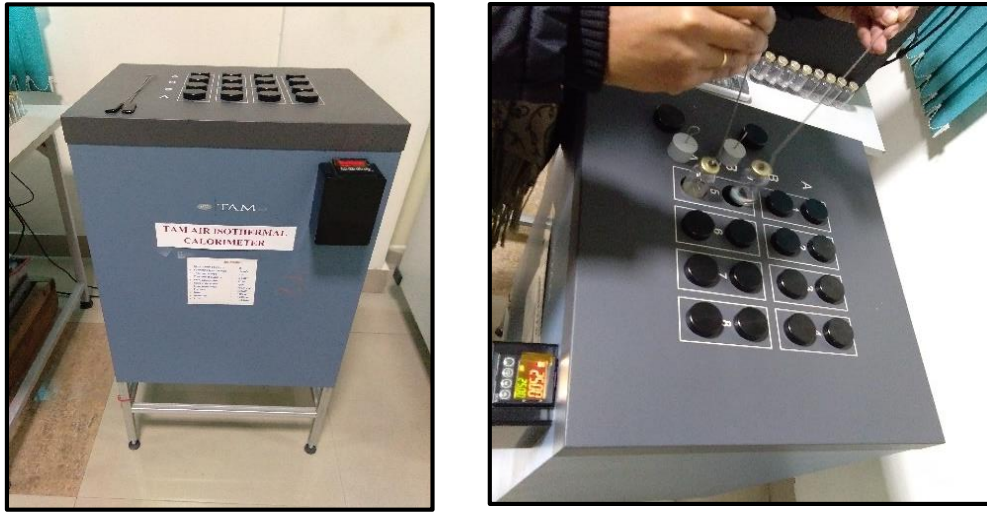
Fig. 3.22: Isothermal calorimeter for hydration kinetics
