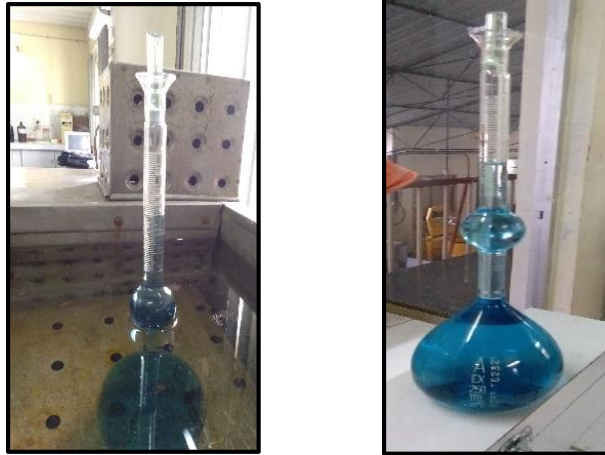
Fig. 3.23: The experimental setup of determining specific gravity of blended cement mixes
