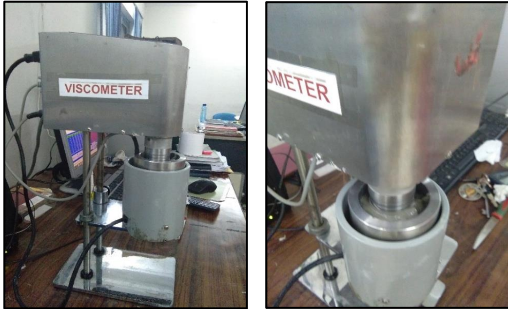
Fig. 3.26: M3500 viscometer for determining rheology of a blended cement paste
