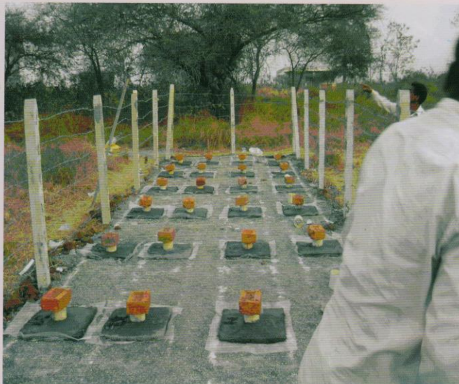
Photo 20 : Modified Ground Board Test at Pune
