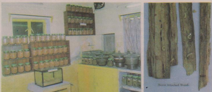
A view of wood-preservative test of materials in BPML (left), and wood-borers and borer attacked wood
