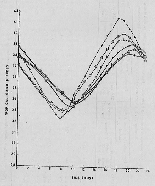
Fig. 1. Comparison of Hourly Variation of Tropical-Summer-Index of 11.5 cm and 23.0 cm Solid Brick Wall Enclosures Under the Three Test Conditions
