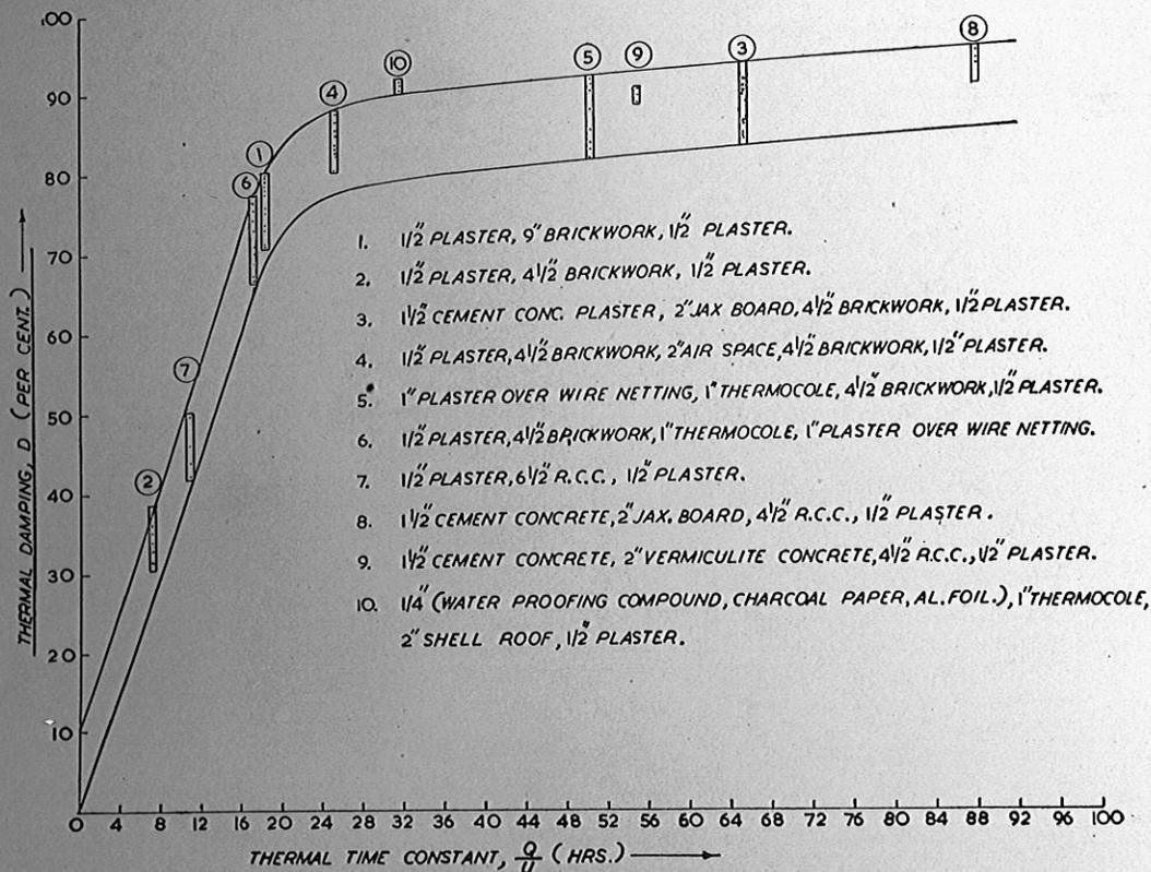
Fig. 3 Thermal Damping, D, caused by panels with different thermal time constants,  $Q/U$ .
