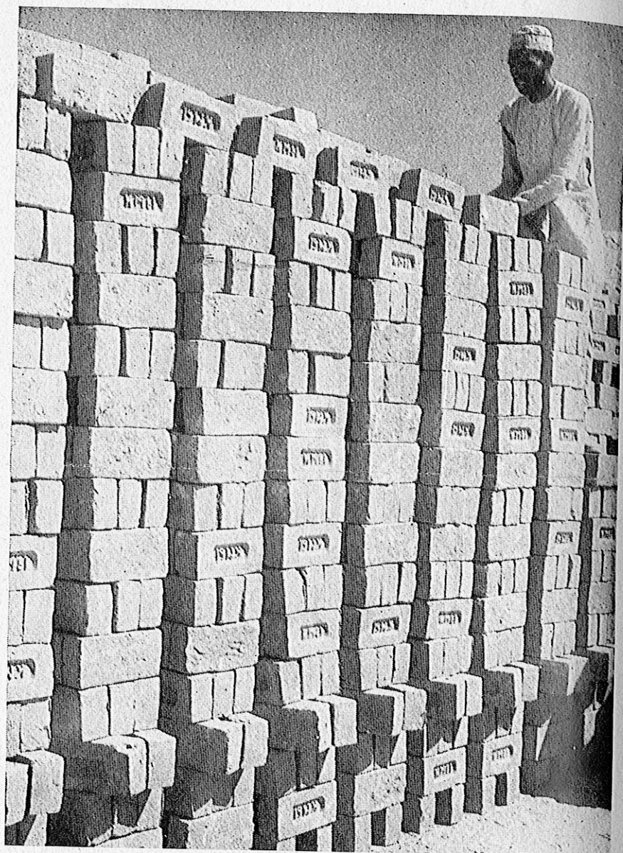
Figure 2. Pattern of setting of bricks in a Bull's Trench Kiln.
