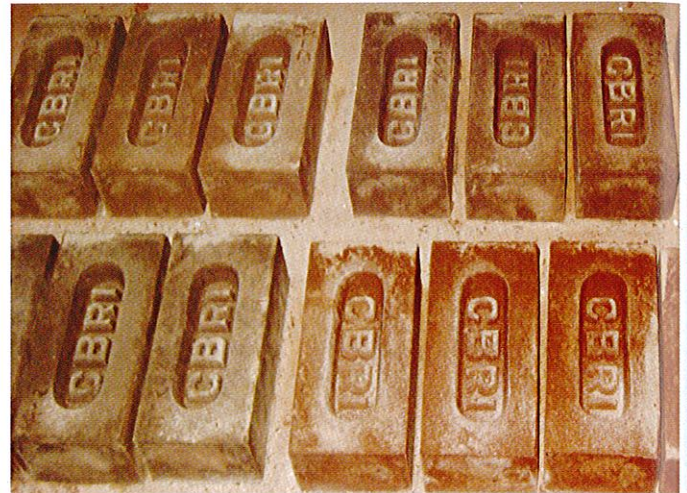
Fig 5: Full Size Green Bricks With Bharuch Soil (20%)
